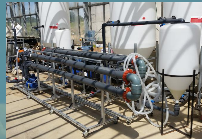
Membrane plant for algal harvesting
