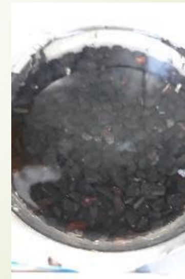
dark coating indicates Mn removal.
