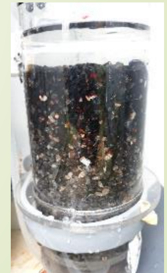
dark coating indicates Mn removal.
