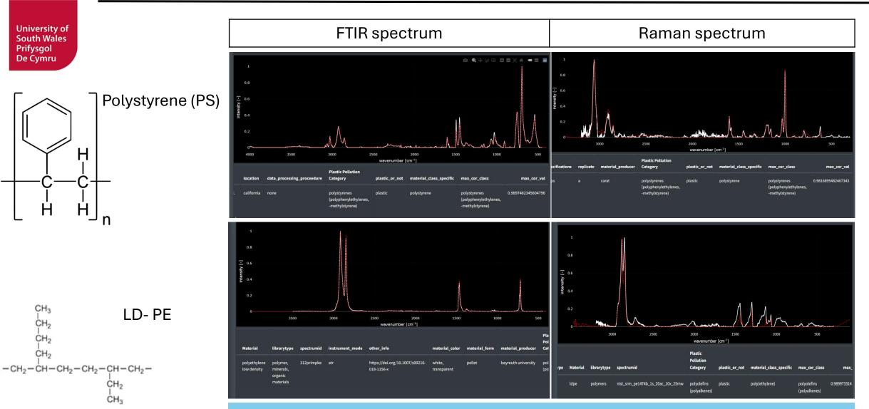
We calibrated 34 standards and aim to analyse them in the samples, with a particular focus on polymers most found in wastewater treatment plants, including those used as flocculants during the treatment process
