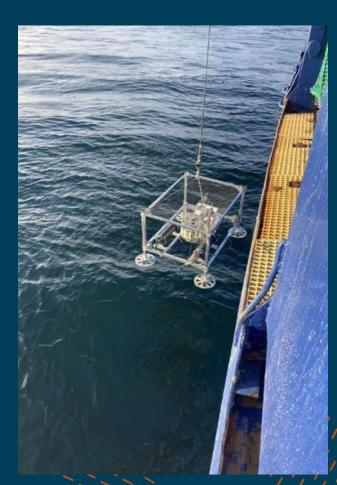
Almost any type of sensor may be attached to a lander (e.g., ADCP, cameras, single-beam or multibeam bathymetry sensors, biochemical sensors etc).
