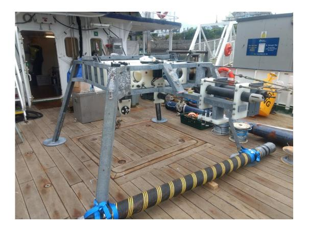
A section of electricity cable was attached to the lander so that on ebb tides turbulent wakes and sediment suspensions from interactions with the cable and frame were measured, and on flood tides a clear boundary layer flow was measured.
