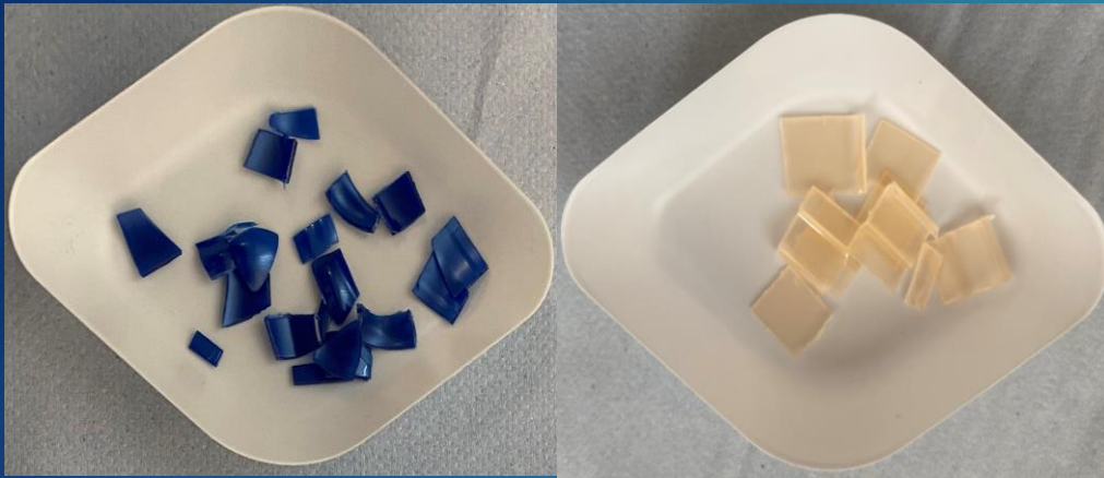
Figure 5. 0.5 g of PCP (left) & food packaging (right) before dry ice & automated homogenization.
