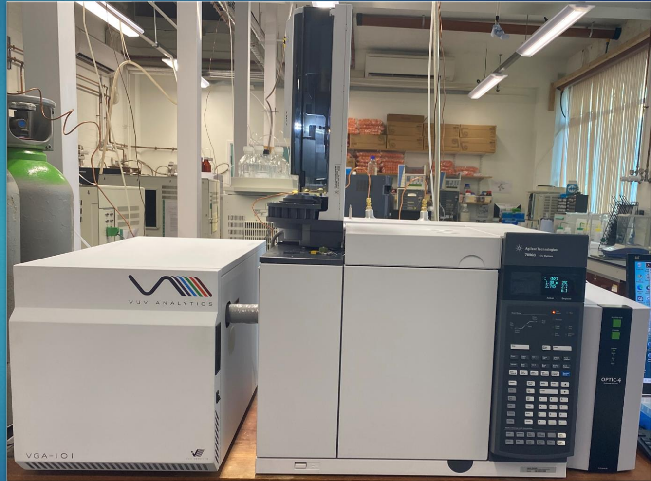
Figure 2. Image of multi-modal GC-VUV, situated in Swansea University's School of Medicine ( 1 st & only in UK! ).
